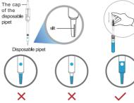
Note 1: Press the top of the disposable pipet to the bottom with your finger during sampling. Ensure that the slit is fully submerged in the sample.
